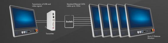
Another advantage is the parallel operation (1:5 operation) via an IPC. Here, up to 5 distance monitors can be operated simultaneously with the help of an extender and an additional switch. The data transmission is also possible with an Ethernet cable up to 100 meters.
